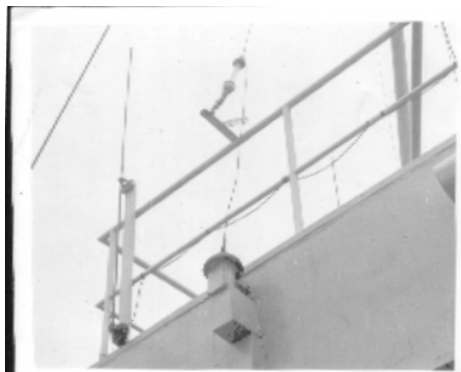
/MM antenna onboard HMS Protector. 10Metre ant on left, inverted 'L' ant when VP8HF/MM.
